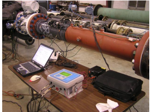
Figure VII. Clamp-On Reference at Custody Meter Calibration
