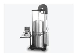
The operation described above assumes that the gas meter is downstream of the bell prover. The
