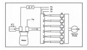
Meter shop provers usually contain between four and seven sonic nozzles, and can vary flow rate between 25 and 2000 cfh. The sonic nozzle prover provides an adjustable table for small and light commercial meter testing, a monitor for interfacing between the prover and the operator, and a state of the art computer enclosure that monitors and controls all proving and data collection operations.
